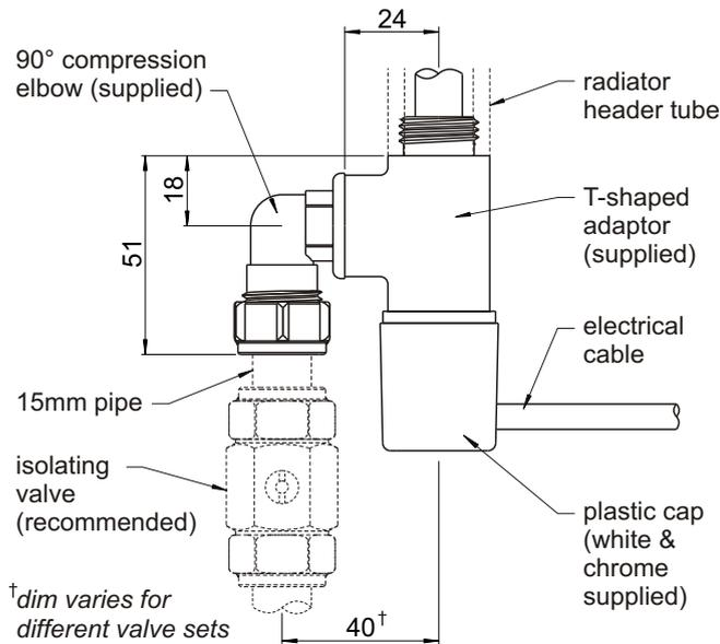
The BTH electric heater should be fitted vertically through the 'T' shaped adaptor supplied and installed on the return side. (See illustration).
